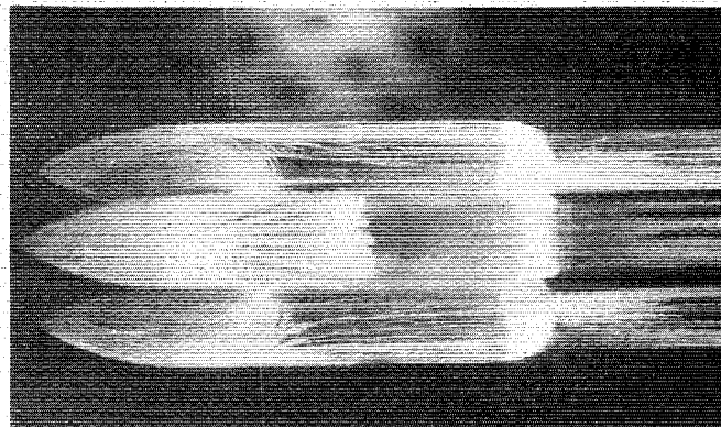
Fig. 12c Triple-store oil flow, M_\infty = 0.95 , \alpha = 6 deg (windward surface).
